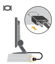
3. Connect the digital cable to the DVI connector of the monitor and the other end on the back of the computer.
